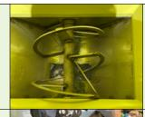
Internal Auger thoroughly mixes and prevents clogging
